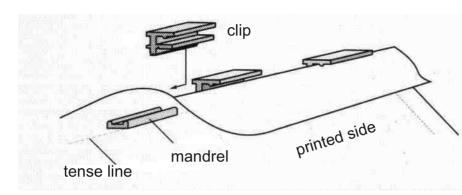
For tensioning of vinyl fabric you have to set the cuts of clips and mandrels of 4 cm, per meter you need 7 to 8 pcs.
