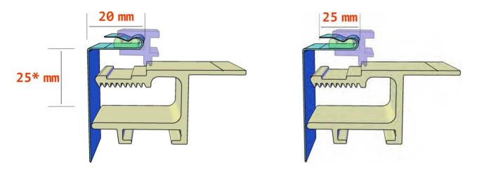
$<sup>^{\</sup>star}$  The visible area rresults of subtracting 25 mm from each outer edge of the fabric sheet.
